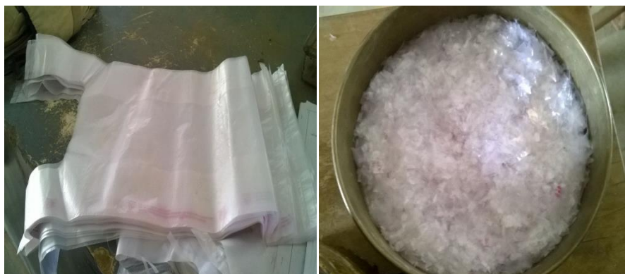
Plastic bag strips used as reinforcement
